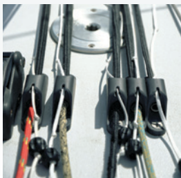
Release lanyard in 'gripping' position
