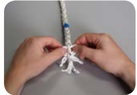
Unlay the rope as far the tape, separating the S and Z strands.
