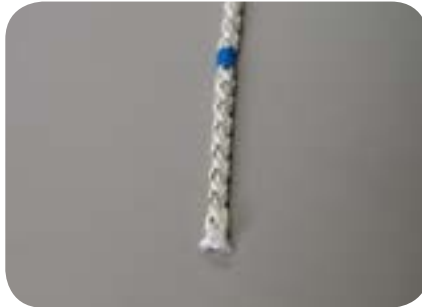
Using a marker pen, mark the first 8 lays and then place a piece of tape.
