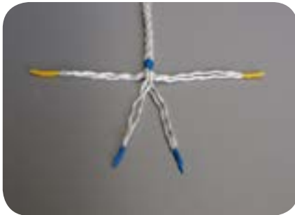
Unlay the S strands, then tape the Z and S strands using different colours.
