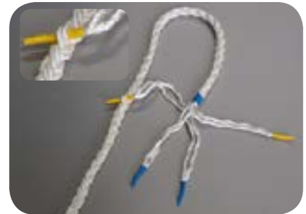
Tuck one of the Z strands under an S strand. The S strands move from left to right, the Z strands do the opposite.
