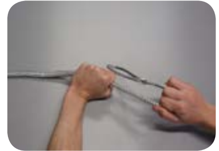
In order to reinsert the end, compact the splice.
