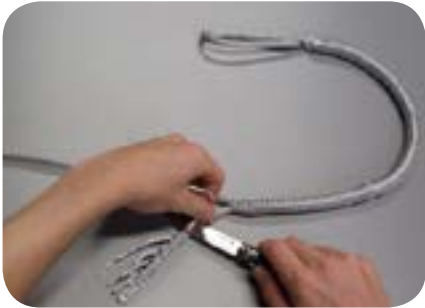
Trim the ends of the strands.
